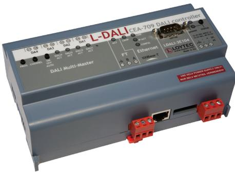
L-DALI controllers are multifunctional devices combining constant light control, sunblind control, and gateway functions between LONMARK and DALI (Digital Addressable Lighting Interface) systems. With alarming, scheduling, trending, and e-mail notification (AST™) the L-DALI Controller is a perfect solution for DALI lighting systems and for a smooth DALI integration into LONMARK Systems.
